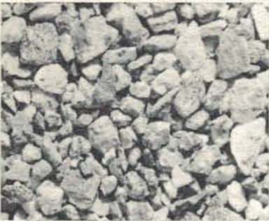
SPCR 3/8 Crushed Rock 300 to 350 lbs. per 100 Square Feet.
