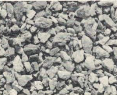
SPCR 1/4 Crushed Rock 200 to 250 lbs. per 100 Square Feet.
