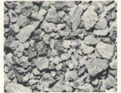
SPCR 3/8 - 1/4 Blend Crushed Rock 250 to 350 lbs. per 100 Square Feet.
